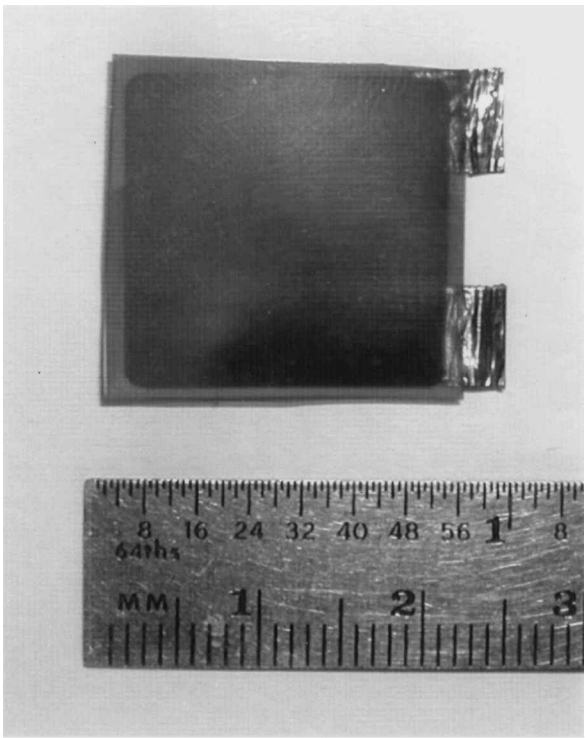
Fig. 9 Solid-state lithium battery (mass-0.5 g).
